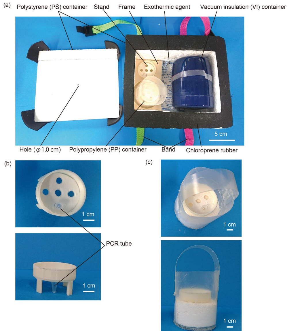
Figure 1. The developed NEC-SD-LAMP device. (a) All components of the NEC-SD-LAMP device. (b) Stand for the SalivaDirect. There are several holes in this component in which to place the PCR tubes. (c) Polypropylene (PP) container. The stands for the PCR tube and palmitic acid are mounted inside this container.
